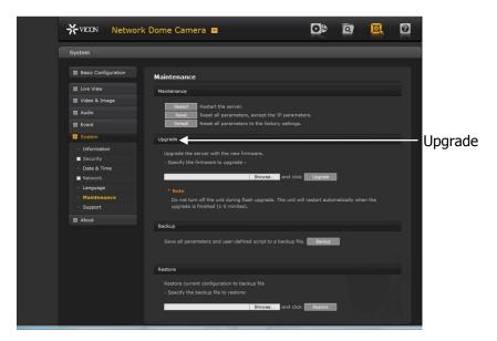
Go to the Upgrade section and use the Browse button to locate the firmware on your PC. Press the Upgrade button. During the upgrade process, so not turn off the power to the camera. Wait at least 5 minutes and access the camera again. The new firmware should be installed. This can be checked from the Basic Configuration screen.
