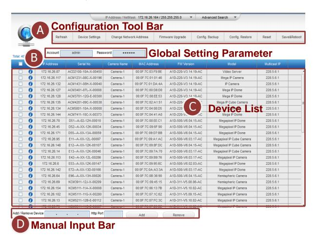
A Configuration Tool Bar: All the functions listed here are configurable through IP Utility.
