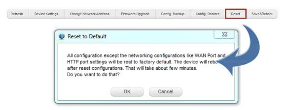
NOTE: The "Save & Reboot" or "Reset" process isn't completed until the device status displays a success message. During this period, please do not disconnect the device.
