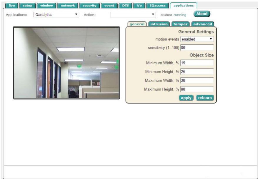
The screenshot displays the IQanalytics web interface. At the top, a navigation bar contains tabs for: **live**, **setup**, **window**, **network**, **security**, **event**, **DTS**, **i/o**, **IQaccess**, and **applications**. Below the navigation bar, the main content area is divided into two sections:
