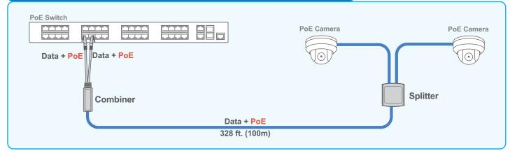
The V-POE-CS2 can connect two cameras at standard UTP distances over a single cable.
