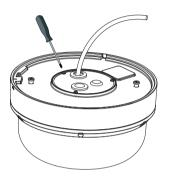
12. Assemble camera with cap first. The  $\bigtriangledown$  should be aligned with OPEN ( \_\_\_\_\_).
