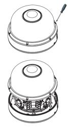
1. Remove and discard the protective EPE from lens modules.
