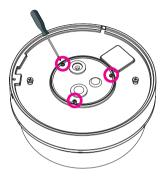
10. Feed the unterminated CAT5 cable through the hole in the solid grommet and terminate the cable with the appropriate connector. If using terminated CAT5 cable, use RJ-45 cap provided to help push the
