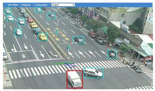
Figure: Wrong Direction Performance On Live View
