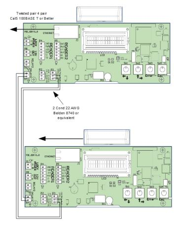
Figure 22.1. Seperate Controller Mantrap
