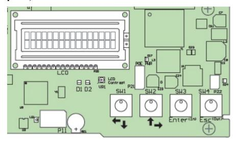
The two white buttons (SW1 & SW2) are used for moving up and down through menus when not editing a specific menu item, and for moving left and right over value data when editing a specific menu item. The two black buttons (SW3 = Enter, SW4 = Esc) are used for selecting a menu item, placing a particular value in edit and non-edit mode, saving or cancelling changes and committing changes to memory.
