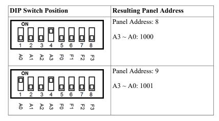
Once you have wired up your **Expander Boards** to the **Elevator Master Panel** and configured the DIP switch **Panel Addresses**, you can now power up the **Elevator Master Board** via 12-13.5VDC power source.
