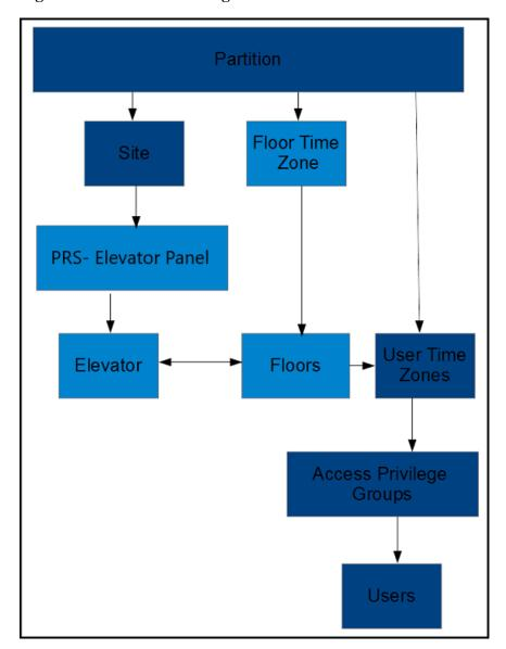
Figure 28.1. Elevator Configuration Items
