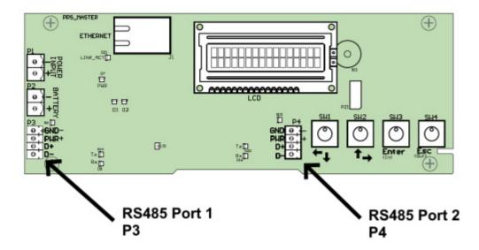
Figure 29.2. OSDP Connection Points (RS-485) on Interconnect Strip
