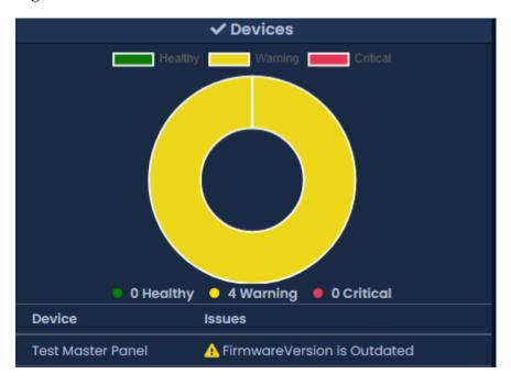
Figure 7.8. Firmware Out of Date Notification
