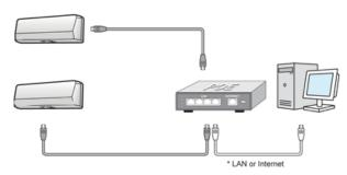
**Controllers - PoE Switch (at Doors) - Router/Switch - PC.** In this scenario the controllers are powered by a PoE switch (above/near the door), which connects (wireless or a single cable) to the site's existing network infrastructure, or an off-site server via an internet connection. This topology is used when it's difficult to run Cat5e to the door, or when the doors are very close to each other.
