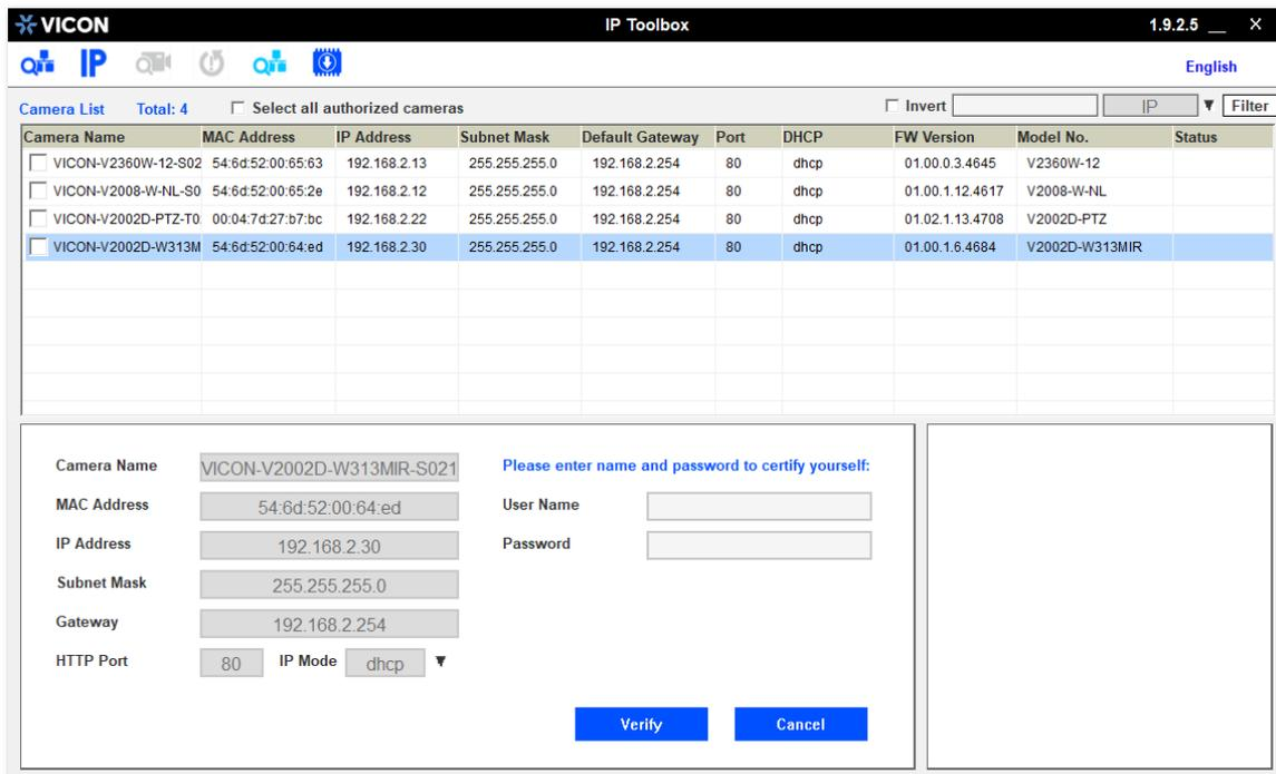
Scan the network to discover the applicable cameras on the local network. Press the firmware update button, select the downloaded firmware and fill in the camera credentials. Press the "+" button, and the list of cameras will appear that are suitable for the selected firmware. (Note that the cameras must have the same credentials, if more than one camera is updated.)
