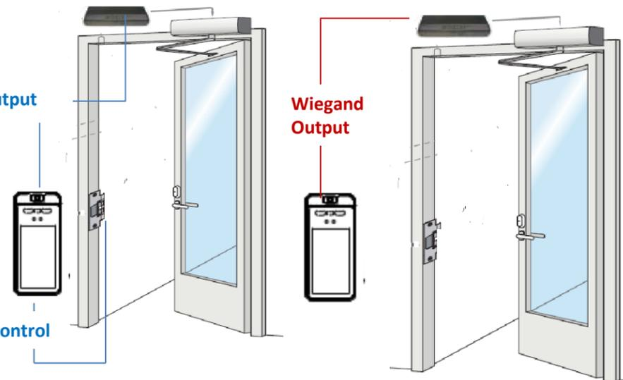
Thermal Biometric Reader can control door locks or activate alarm outputs
