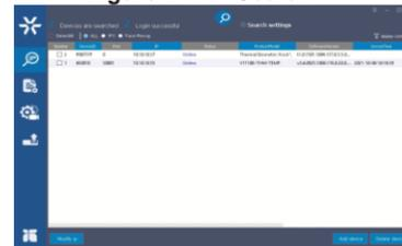
Click icon to find all the current cameras. Click the camera to configure. Click "Modify ip" and select DHCP to assign IPs or Static to enter the values.
