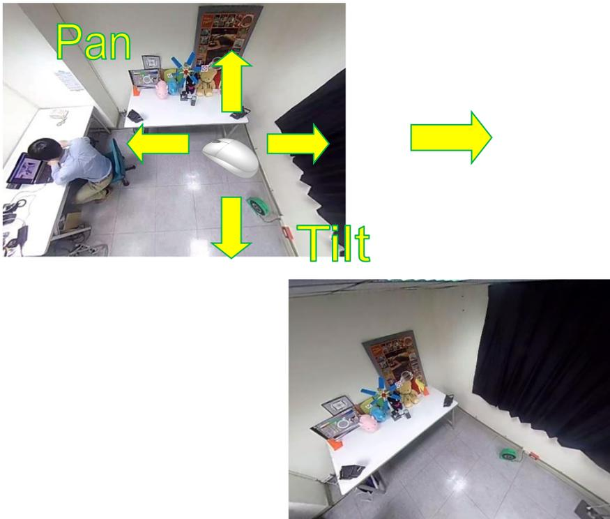
Figure: ePTZ Pan and Tilt Manipulation
