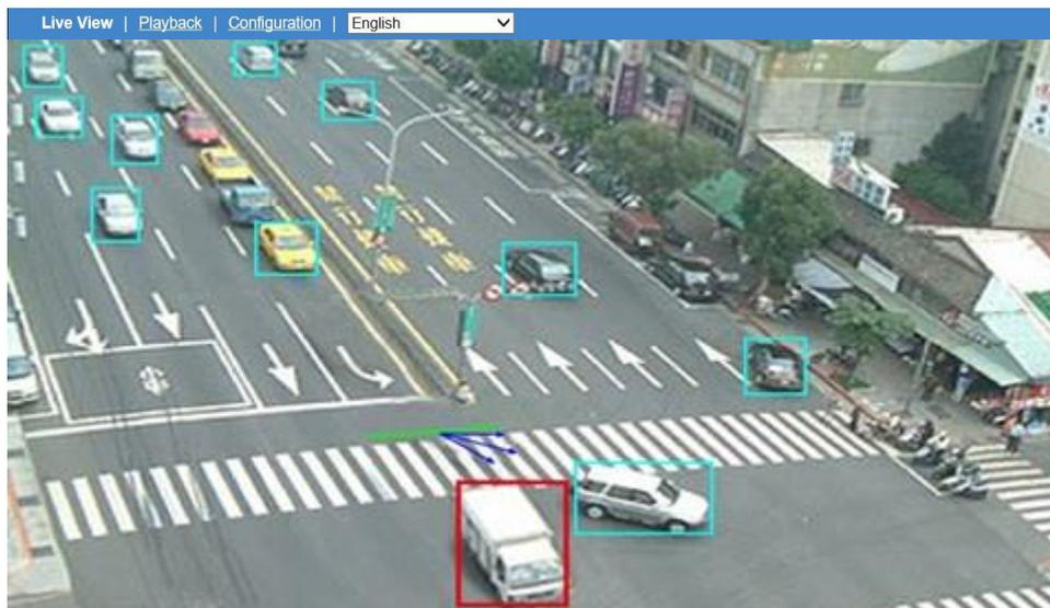
Figure: Wrong Direction Performance On Live View
