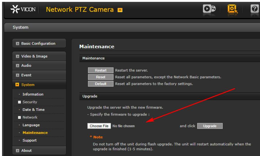
Open the Upgrade section and use the Browse button to locate the firmware on your PC. Press the upgrade button. During the upgrade process, do not turn off power to the camera. Wait at least 5 minutes and access the camera again. Once complete, the firmware version can be checked on the Basic Configuration screen.
