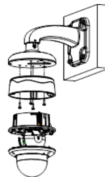
FIGURE 3-2: SECURE VANDAL DOME CAMERA ON THE BRACKET
