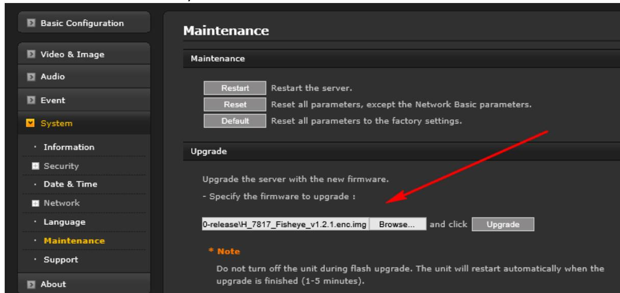
Open the Upgrade section and use the Browse button to locate the firmware on your PC. Press the upgrade button. During the upgrade process, do not turn off power to the camera. Wait at least 5 minutes and access the camera again.
