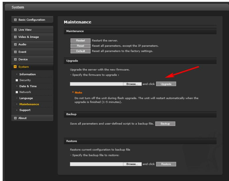
Open the Upgrade section and use the Browse button to locate the firmware on your PC. Press the upgrade button. During the upgrade process, do not turn off power to the camera. Wait at least 5 minutes and access the camera again.
