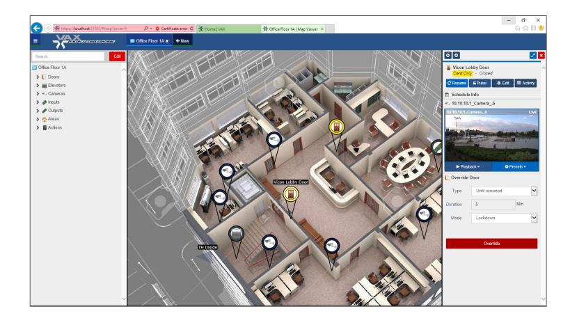
Set icons for a door, elevator, input, or output allow you to see the real-time state (e.g., Card Only access) of that object, associated video, and gives you Override control
