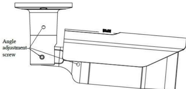
Figure 2-4 Adjust the camera angle
