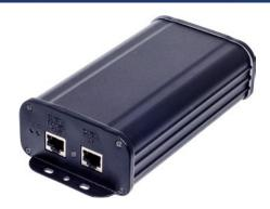
The HPOE-70W-INJ is a UPoE injector that uses the same cabling standard as PoE. Instead of delivering power over two twisted pairs, it provides the capability to source up to 60W of power by using all the four pairs of standard Ethernet cabling (Cat5e or better).
