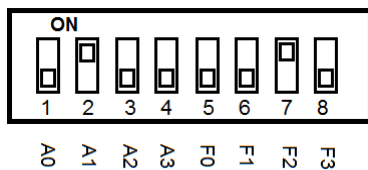
Figure 27.5. DIP Switch: Tamper Sensor
