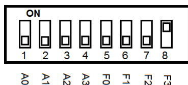
Figure 29.4. DIP Switch: Input/Output Test
