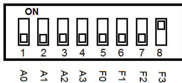
Figure 27.4. DIP Switch: Input/Output Test
